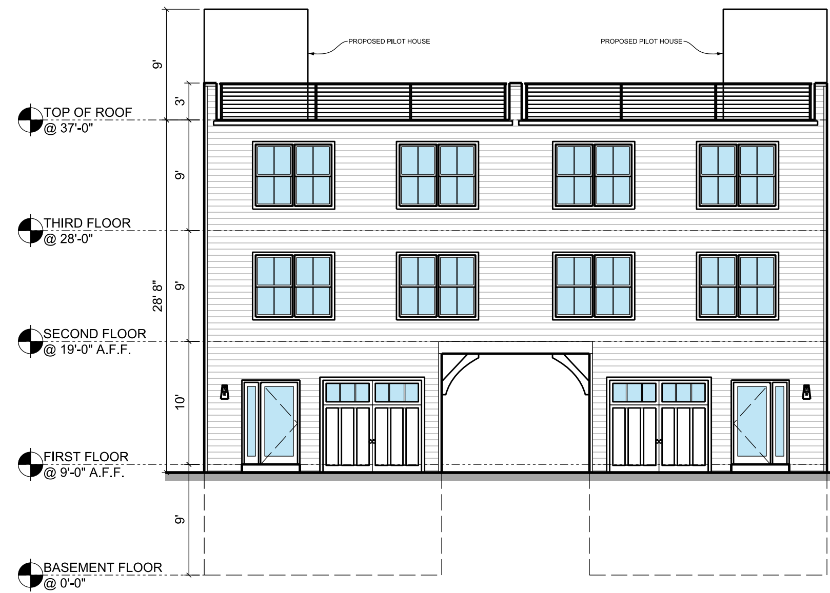
3/Z-002 PROPOSED SIDE ELEVATION - PARCEL C 3/16" = 1'-0"
