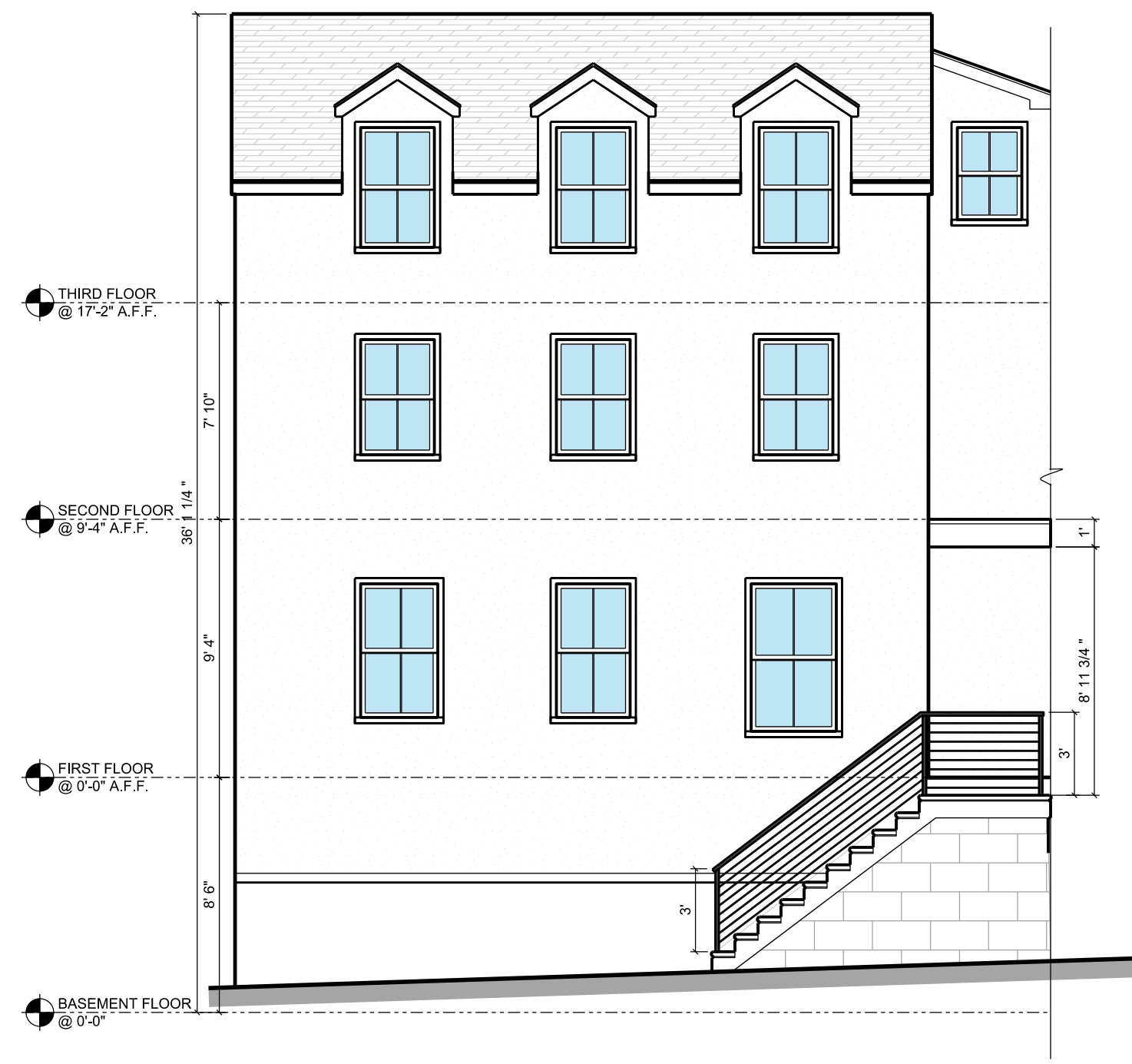
1/Z-002 PROPOSED FRONT ELEVATION - PARCEL C 3/16" = 1'-0"
