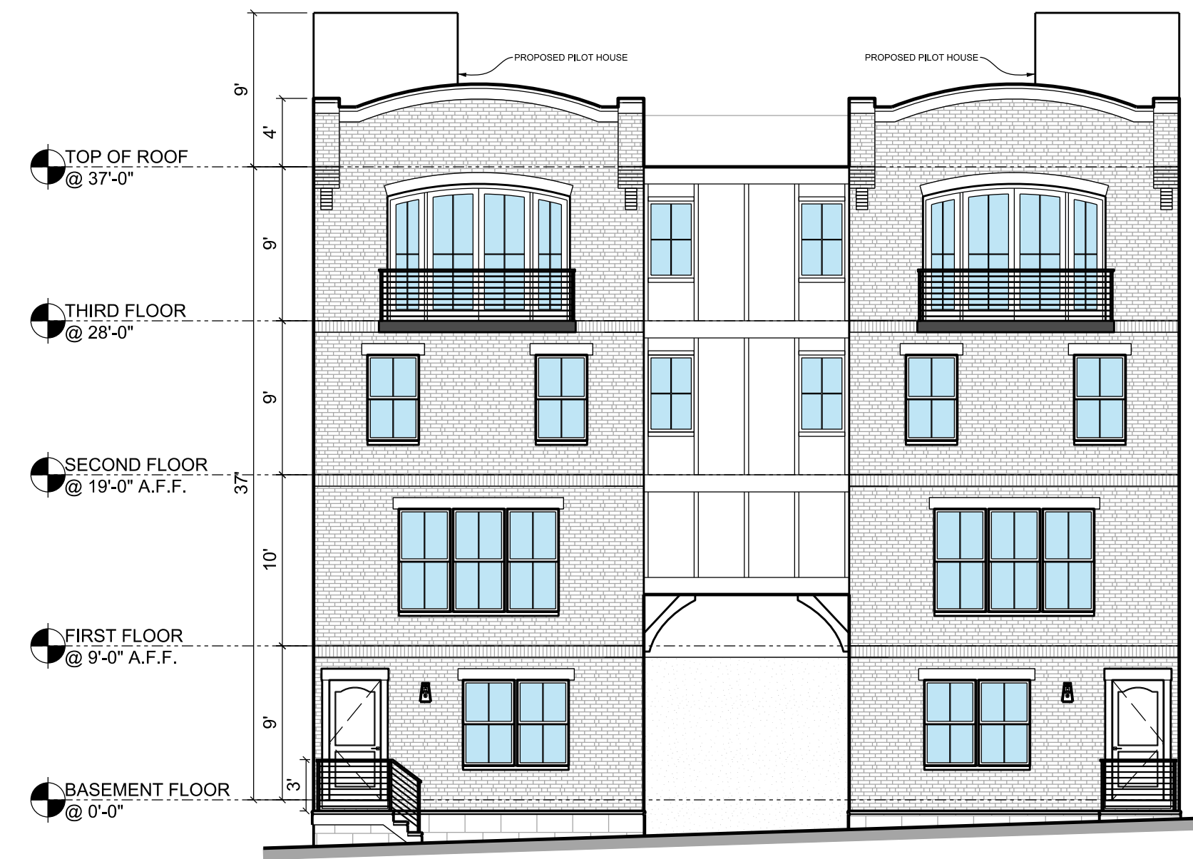
4/Z-002 PROPOSED FRONT ELEVATION - PARCEL A & B 1/8" = 1'-0"
